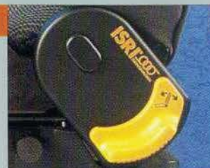
Backrest adjustment, in fine increments, 2°
